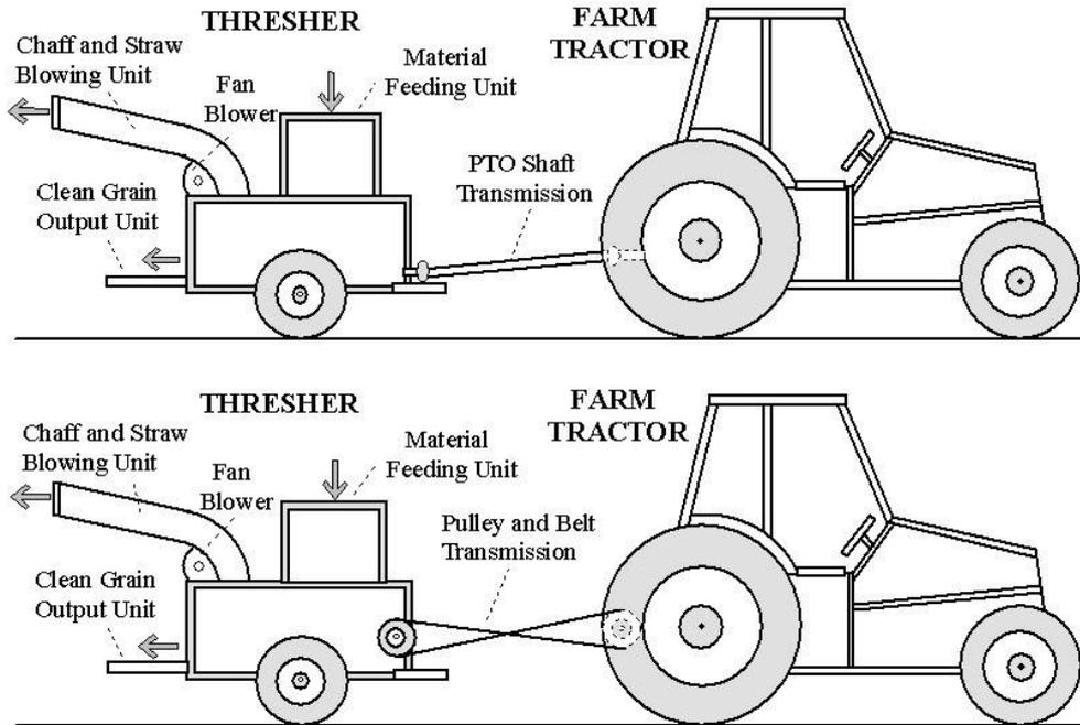
Figure 1. Threshers powered by tractor PTO shaft (top) and pulley system (bottom)
